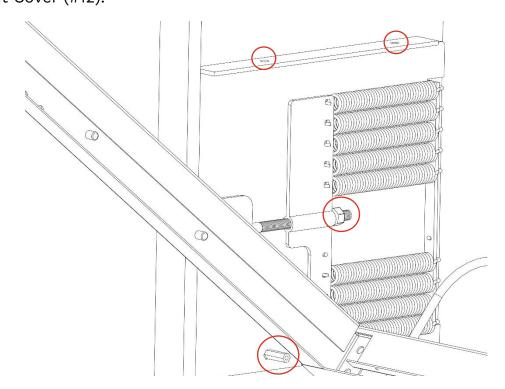
Tightening the tension will lighten the load making it easier to lift especially with a heavy mattress. Loosening the tension will make it less springy and heavier.
