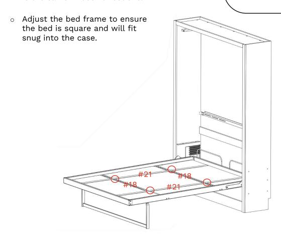
Standard measurement for a Queen Vertical Embed is 103 1/4" corner to corner
